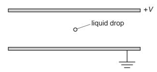
A small charged liquid drop, midway between the plates, is held in equilibrium by the combination of its weight and the electric force acting on it.
